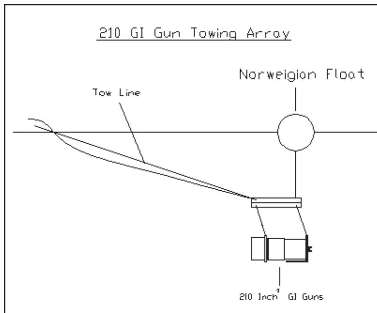
Figure 6.8 GI Gun towing configuration during Hudson 2008-029
