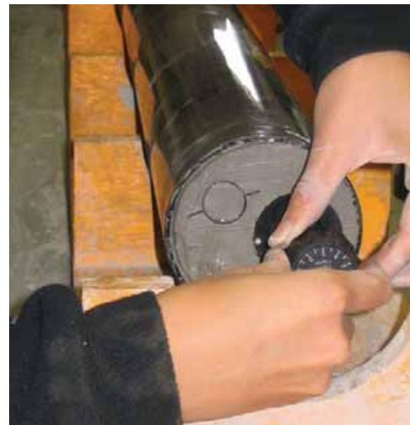
Figure 6.4 Taking a Torvane measurement.
