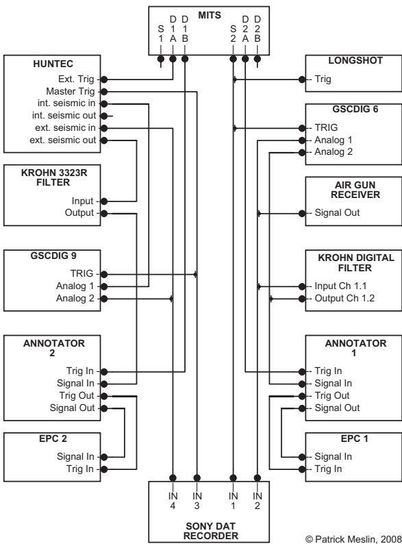
Figure 6.11 Electronics wiring diagram during Hudson 2008-029
