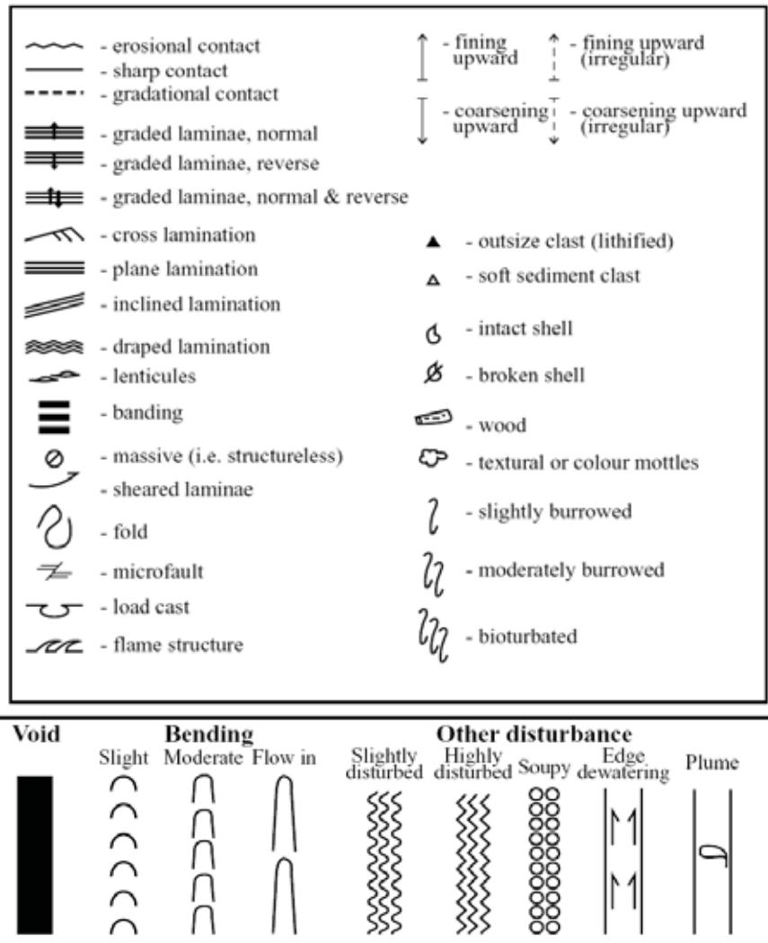
Figure 6.6 - Symbols used to characterize the sedimentary structures and coring disturbances
