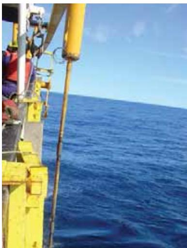
Figure 6.1 Recovering the Piston Corer.
