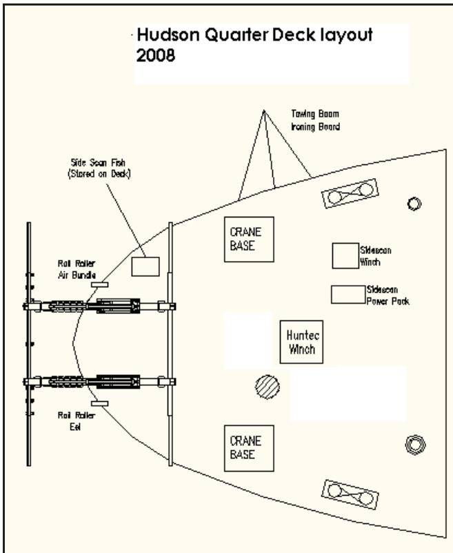
Figure 6.9 Quarter deck layout during Hudson 2008-029
