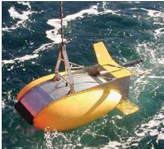
Figure 6.12 Huntec DTS being deployed
