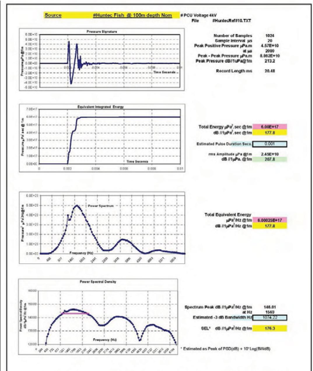
Figure 6.14 Calibrated source signature data for Hunttec DTS sparker.
