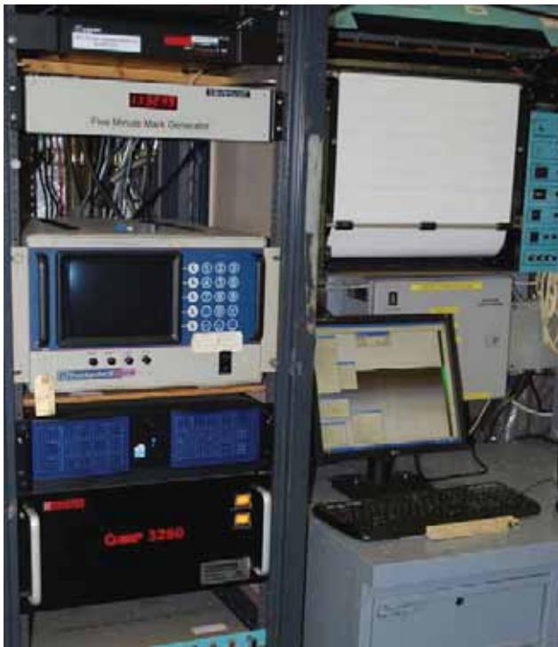
Figure 6.15 Knudsen chirp console and logging
